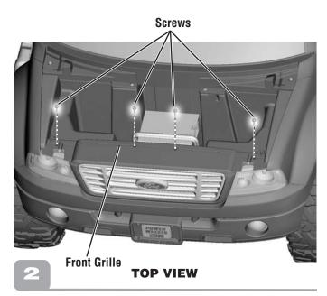
• Insert four screws into the top of the front grille and tighten. *Hint:* You may need to push the ends of the front grille to insert and tighten the outer screws and push the center of the front grille to insert and tighten the middle screws.
